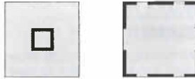
Stabilizing elements may be placed within the interior or at the perimeter of a building.
